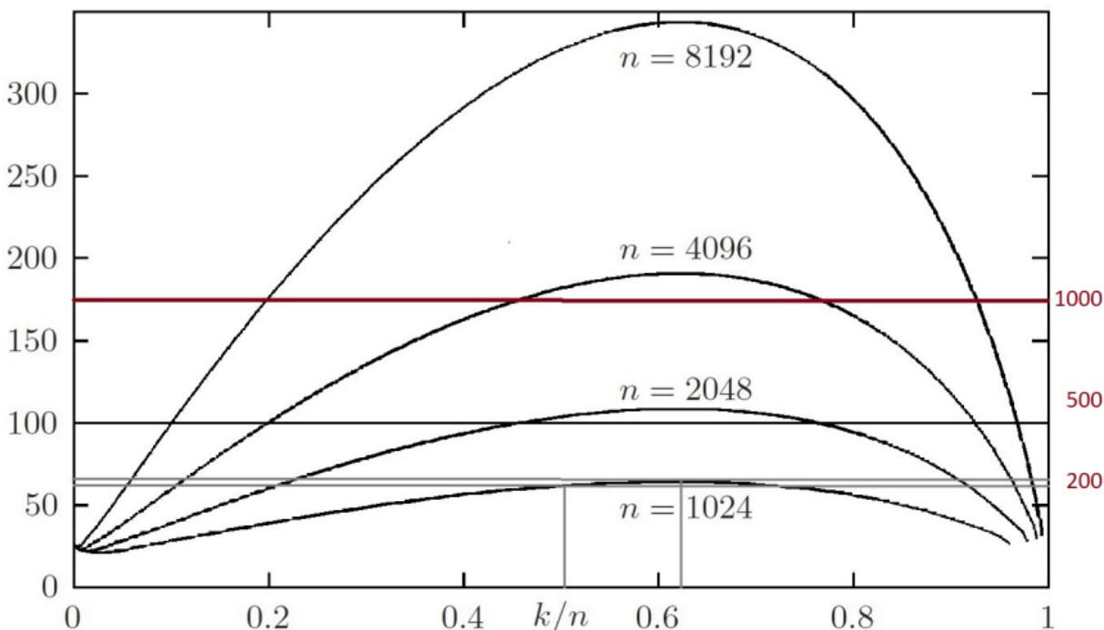
Horizontal axis  $R = k/n$ , WF curves for  $n = 2^j$ ,  $j = 10, \dots, 13$ . The red line represents the WF needed to break RSA with 1000-digit prime numbers. The similar 500-digit and 200-digit levels are also shown. The latter is comparable to the original McECS.
