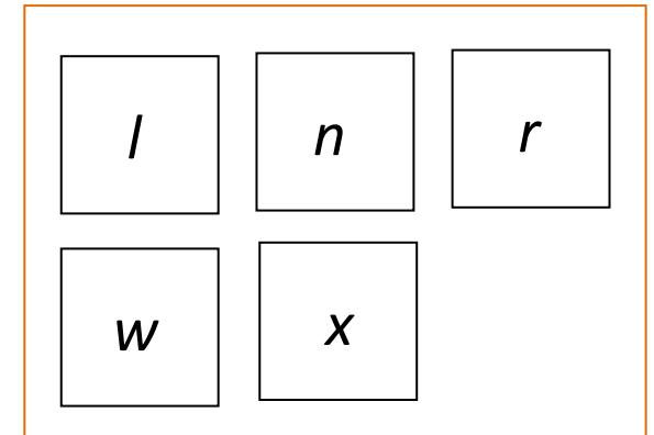
$$\hat{x} = \begin{cases} \max(w, n) & \text{if } \max(n, w) \leq l \\ \min(w, n) & \text{if } \min(n, w) \geq l \\ n + w - l & \text{otherwise} \end{cases}$$
