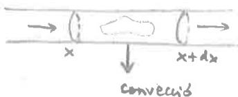
$$-\beta(x) \cdot (T(x,t) - T_{\infty}(x,t)) \underbrace{p(x) dx dt}_{\text{dens. flux de converg\acute{e}e}} \underbrace{\text{\'{a}rea sup. lateral}}_{\text{dens. flux de converg\acute{e}e}}$$
