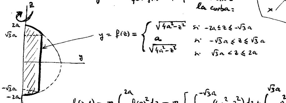
$$y = f(z) = \begin{cases} \sqrt{4a^2 - z^2} & \text{si } -2a \leq z \leq -\sqrt{3}a \\ \frac{a}{\sqrt{4a^2 - z^2}} & \text{si } -\sqrt{3}a \leq z \leq \sqrt{3}a \\ \sqrt{3}a & \text{si } \sqrt{3}a \leq z \leq 2a \end{cases}$$
