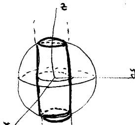
$$\begin{aligned} \text{vol}(W) &= \pi \int_{-2a}^{2a} f(z)^2 dz = \pi \cdot \left[ \int_{-2a}^{-\sqrt{3}a} (4a^2 - z^2) dz + \int_{-\sqrt{3}a}^{\sqrt{3}a} \frac{a^2}{4a^2 - z^2} dz + \int_{\sqrt{3}a}^{2a} (4a^2 - z^2) dz \right] = \\ &= \pi \cdot \left[ 2 \cdot \left( \frac{16}{3} - 3\sqrt{3} \right) a^3 + 2\sqrt{3} a^3 \right] = \underline{\underline{\frac{4\pi}{3} \left( \frac{8}{3} + \sqrt{3} \right) a^3}}. \end{aligned}$$
