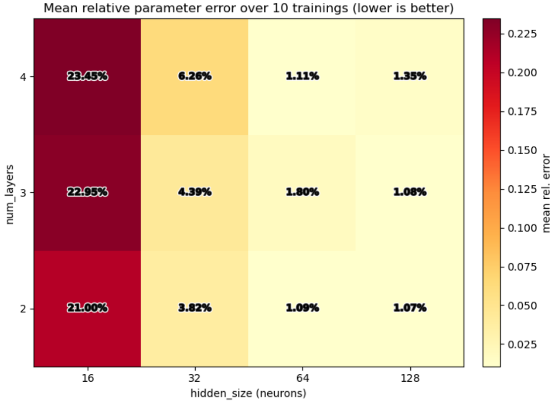
Figure 5: The architecture with two hidden layers and 128 neurons was chosen because it provided the best trade-off between model complexity and parameter identification accuracy, achieving the lowest average relative error among all tested configurations.
